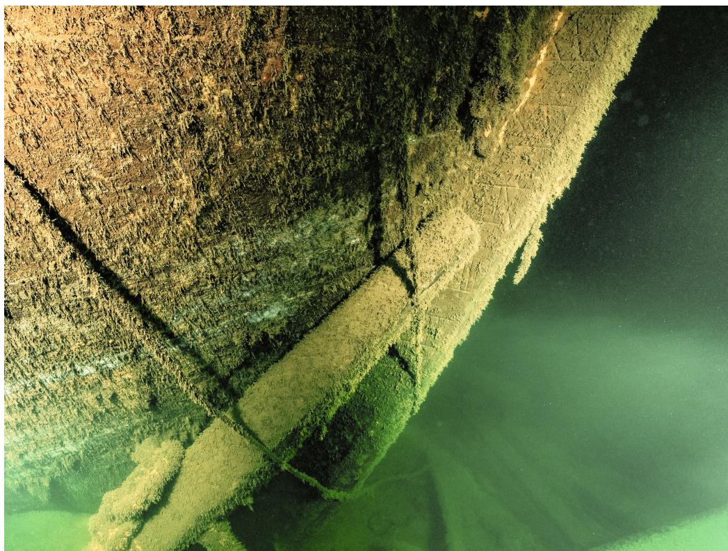
Fig. 2. Carved depth marking on the stempost.
