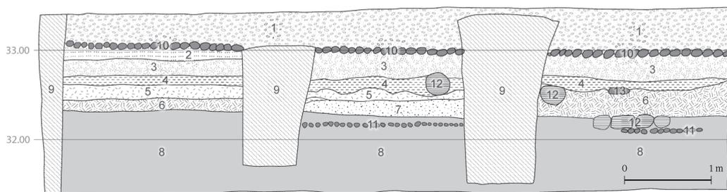
**Fig. 2.** Section of the wall of the pipeline installation in front of Kivi Street 40a. 1 – crushed stone, 2 – brown sand, 3 – yellow sand, 4 – red sand, 5 – mixed fill soil rich in humus, 6 – fill of mixed soil and sand, 7 – grayish sand, 8 – 16th – 18th century cultural layer, 9 – filling sand, 10 and 11 – cobblestone pavements, 12 – wood.
